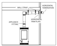
Figure 7- Double Wall Horizontal
