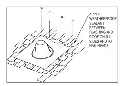
Figure 14- Flashing
