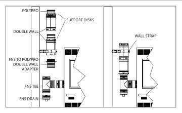
Figure 6- Horizontal Appliance Outlet
