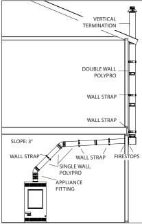
Figure 8- Single Wall / Double Wall
