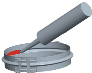
Figure 6 - Joint Assembly Step 1
