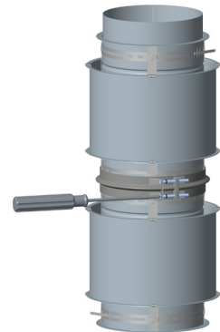
Figure 9 - Joint Assembly Step 4
