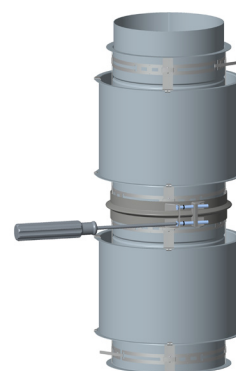
Figure 9 - Joint Assembly Step 4
