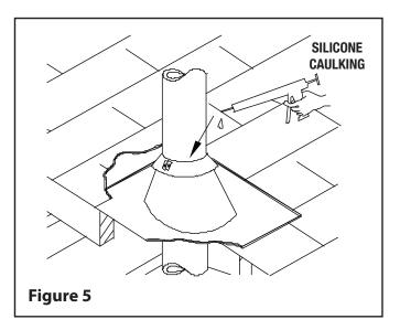
Step 9: Tighten the collar using the supplied bolt. Make sure the joint is properly caulked (see Figure 5).
