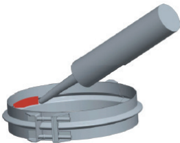
Figure 12: Joint Assembly Step 1
