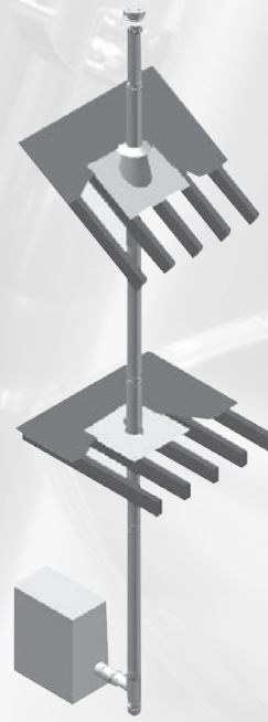
DuraSeal Double Wall (DSD) Vertical Through-the-Roof Installation
