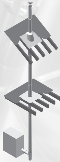
DuraSeal Double Wall (DSD) Vertical Through-the-Roof Installation
