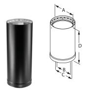
Designed for installation with minimum clearance to combustibles (6" to walls, 8" from top of horizontal run to ceiling). Available in 6", 7", and 8" diameters. Subtract 3/4" for installed length. Constructed with a stainless steel inner wall.
