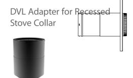
This adapter is similar to our current DVL adapter but has a longer inner sleeve and an additional wrapping outer sleeve. Longer inner sleeve enables adapter to be used on short stove collars as well as on stove collars with nearby interfering features, like a convection deck. Wrapping outer sleeve conceals coupling between stove and adapter, and enables user to install on stoves with collars up to 4 inches tall.
