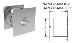
Use for through-the-wall termination. Fits between standard wall studs. 3''-5'' diameters accommodate wall thickness of  $4 \frac{1}{2}$ " to  $8 \frac{1}{2}$ ". 6''-16'' diameters accommodate wall thickness of  $5 \frac{3}{4}$ " to  $11 \frac{1}{2}$ ".
