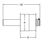
Use for through-the-wall termination. Fits between standard wall studs. 3''-5'' diameters accommodate wall thickness of  $4 \frac{1}{4}''$  to  $8 \frac{1}{2}''$ . 6''-16'' diameters accommodate wall thickness of  $5 \frac{3}{4}''$  to  $11 \frac{1}{2}''$ . AVL pipe allows for adjustability in length variance.
