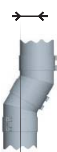
Figure 28 – MINIMUM OFFSET for ELBOWS
