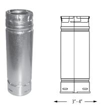
Features fully unitized, twist-lock construction in 3" and 4" diameters. Listed at 1" clearance to combustibles. It can be used in both vertical and horizontal installations. Stainless steel wall combined with a galvanized outer wall. Pipe OD is diameter plus %". Galvalume or painted black outer finish. 12" length available with stainless steel outer (SS).
