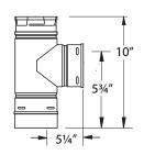
Attaches 3" pipe to branch and 4" pipe to body. Use for a 90° offset. Branch swivels for alignment. Removable twist-lock Clean-Out Tee Cap.
