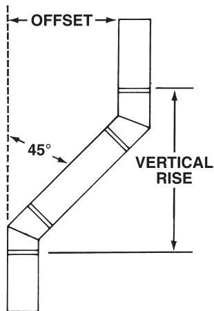
**Note:** The vertical rise can also be closely estimated by adding one "A" and one "B" dimension to Maximum Offset figures. (See page 14 for "A" and "B" dimensions of Round Adjustable 45° Elbows.)
