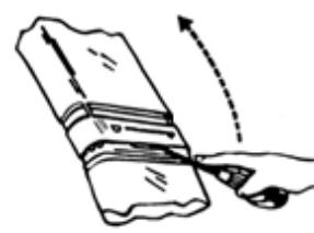
Press firmly inward with blade of screwdriver and pry upwards VERY SLOWLY AND GENTLY. Joint will slowly separate without damage.
