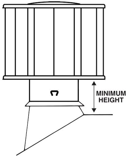
Caps in 3" through 12" sizes may be installed in accordance with the Gas Vent Termination Table if the vent is at least 8' from any vertical wall.
