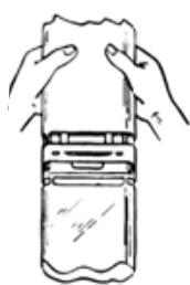
Press side of pipe down until joint seats.
