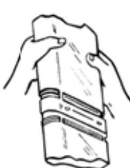
Press other side of pipe down until joint is engaged.
