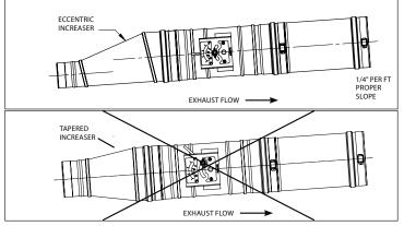
Note: Damper can be installed Vertically, Horizontally, and Diagonally. Consult installation manual for details.
