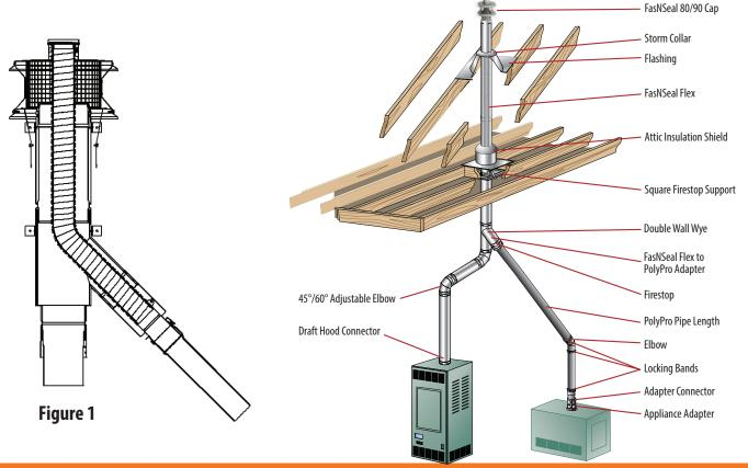
The exhaust streams from the atmospheric water heater and the condensing furnace never mix. Rather, all of the exhaust from the furnace is contained within the stainless-steel flex, while the exhaust from the water heater is contained within the space between the flex and the B vent.
